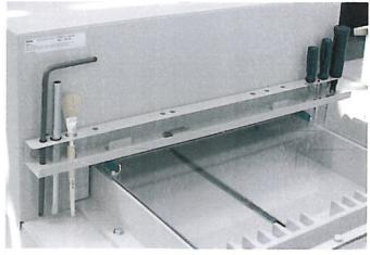
HOOK-IN TOOL HOLDER The practical hook-in tool holder is placed on the back table and keeps all necessary tools for blade change and service jobs within reach.
