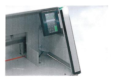
IR LIGHT BEAM SAFETY CURTAIN Efficient and safe cutting and trimming is guaranteed by the IR light beam safety curtain on the front table.
